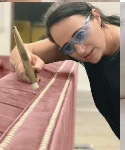
OUR CRAFTSPEOPLE COMPLETE EACH SHELTON WITH NAILHEADS, USING A MALLET TO WORK EACH NAIL INTO THE FRAME-ONE AT A TIME, IN PERFECT ALIGNMENT.
